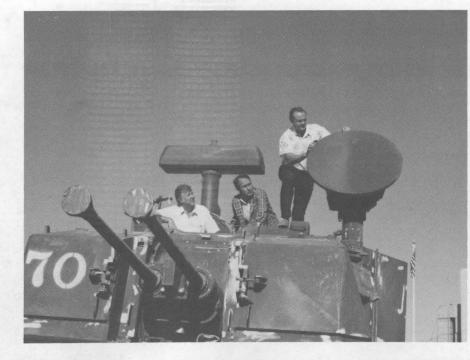
RADAR SYSTEM on one of the York guns is checked at the Tonopah Test Range by (from left) Carl Smith (7174 supervisor), Jerry McCorkle (7174), and TTR manager Ron Bentley (7170). The sophisticated radar system is the same type used on the advanced F-16 fighter aircraft ---the Fighting Falcon. The round unit that Ron is checking is a targeting radar; the rectangular unit is a surveillance radar. One of the uses planned for TTR's Yorks is mobile radar tracking of targets.
